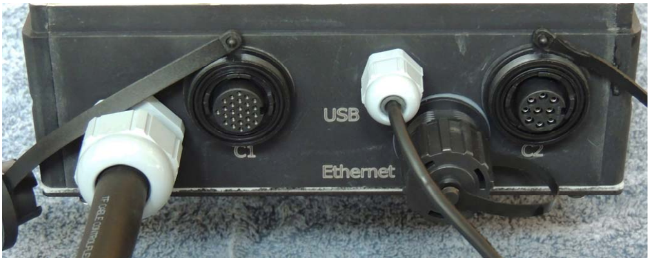
Figure 11. LDR Laser Head Rear Panel Connectors
