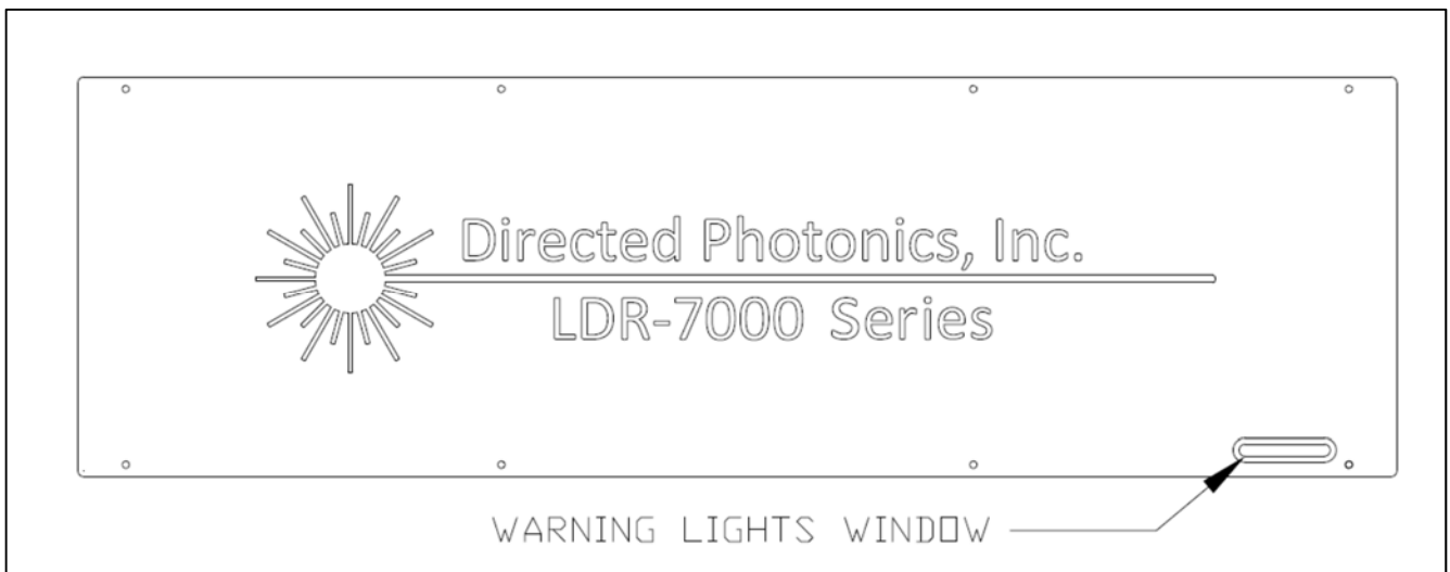
Figure 2. LDR Warning Lights Window Location
