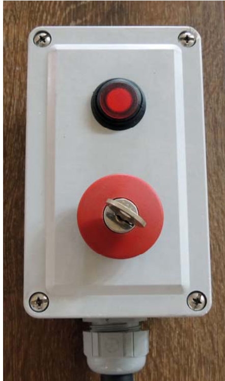
Figure 1. LDR Control Pendant with E-Stop/Key-Switch and Arming Switch
