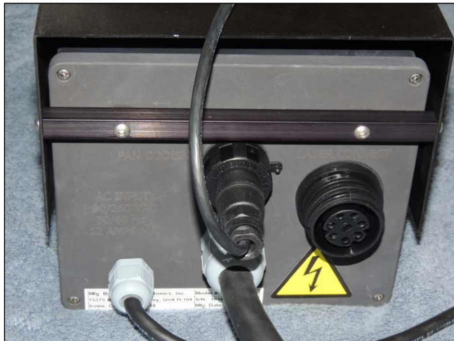
Figure 17. LDR Power Supply Module (Front View)
